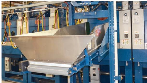
Milnor dryers are pass-through machines that load at one end and discharge at the other. They form an integral part of an automated batch laundry processing system, along with a PulseFlow<sup>®</sup> batch washer or continuous batch washer, an extraction system, and transport conveyors.
